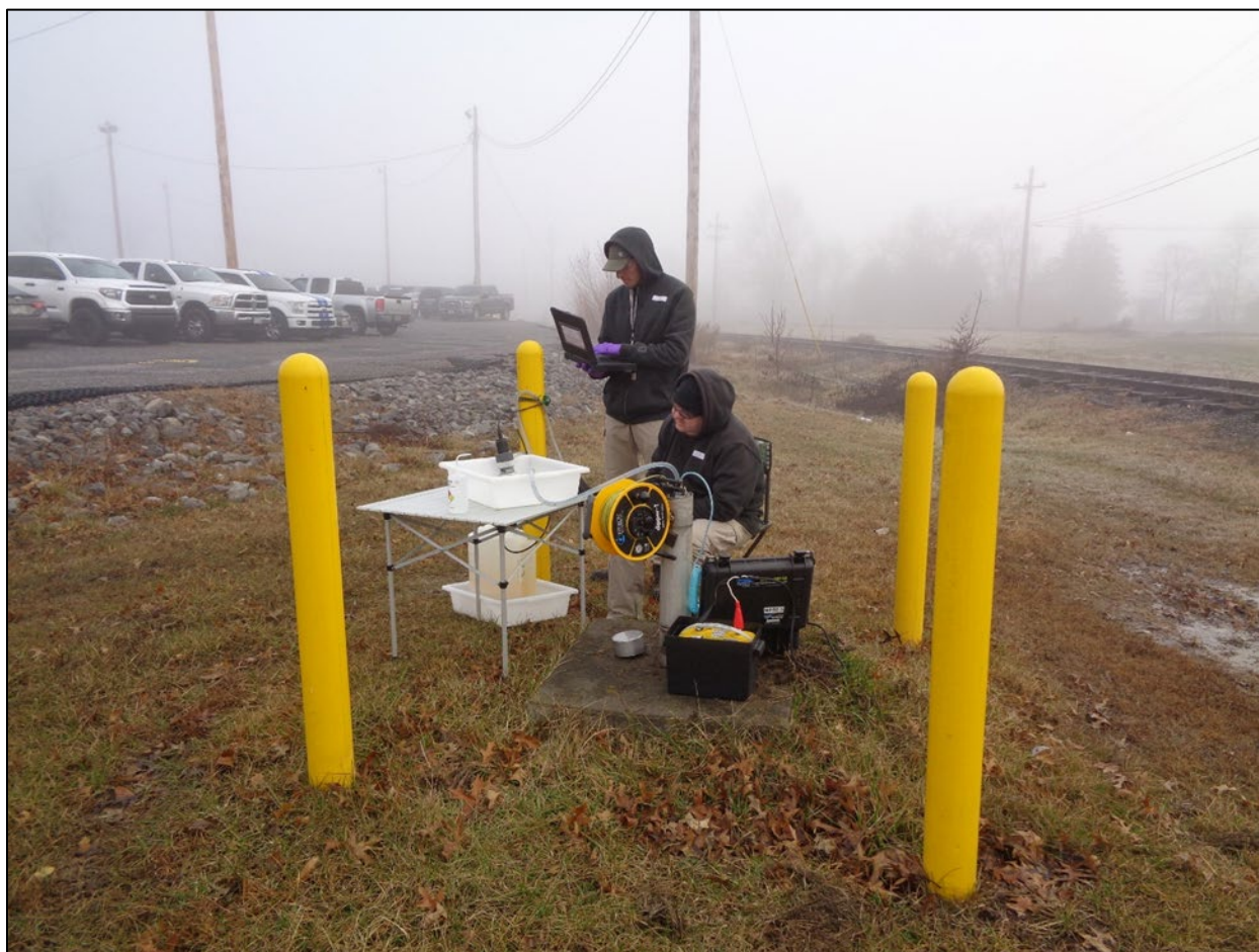
Figure 4.28. Groundwater monitoring well sampling at Y-12
